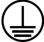
When supplying power to this equipment, connect the accessory 3-pin power cord to a 3-pin grounded power outlet. If required, ground the instrument chassis to a suitable earth ground. If power is supplied without grounding the equipment, there is a risk of receiving a severe or fatal electric shock.
