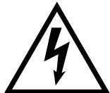
This equipment may present a risk to electric shock. Only qualified service personnel should access areas where this alert mark is present. Ensure that precautions are taken and that appropriate lockout mechanisms are in place before proceeding to enter the areas presenting this risk.
